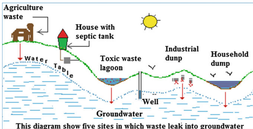
Fig. 1.5 Transformation of waste leakage into groundwater
